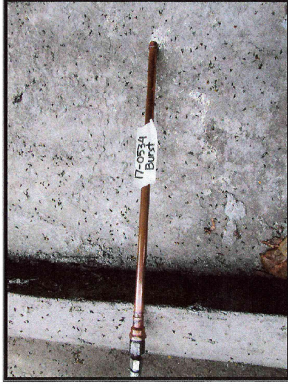
Test set-up for the Burst Test of Copper Tube: 5/8" Ø
